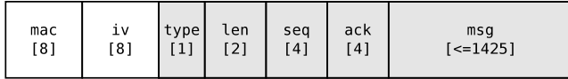
Figure 4: SkypeMorph UDP packet body layout, where the size (in bytes) is under the name for each field. The shaded parts are encrypted using 256-bit AES counter mode. All bytes after the mac field are included in the HMAC-SHA256-64 computation.
